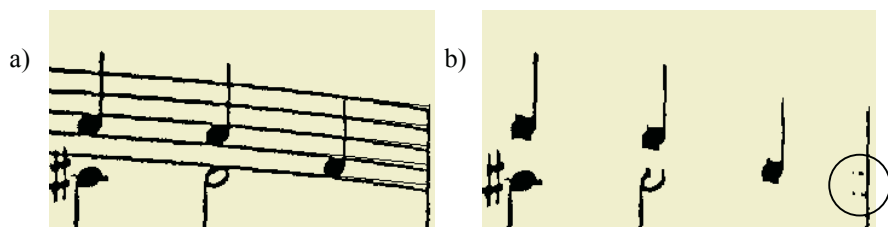
Fig. 7. An example of staff lines' approximation errors: a) part of original image with approximating cubic curves and b) staff lines removing errors (circled)
