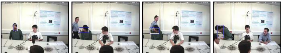
Fig. 1. Head tracking using CamShift. Frames #10969, #11224, #11233, #13669.
