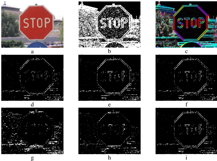
Fig. 5. Detection of the “B20” (STOP) sign: color image (a), structural places (b), HSI representation of components T_{ij} (c), detected silhouettes for different sets of c_i (d-i)
