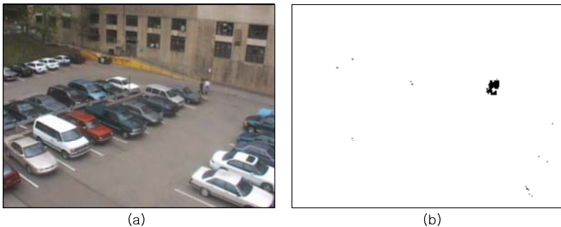
Fig. 1. Target people in a low-resolution image: (a) Original image, (b) Foreground detection
