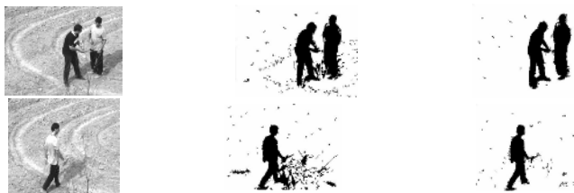
Fig. 4. The results obtained applying to a pair of images a traditional statistical background modelling [3] (2 nd column) and the proposed algorithm (3 th column)
