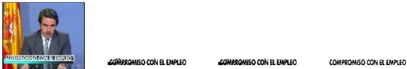
Fig. 4. The extraction results. From left to right: (a) the result of the localization alg. in [7]; the segmentation results (b) using Otsu [16]; (c) using k-means [9]; (d) using the proposed AFTS.
