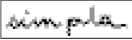
Fig. 1. Order dependent (dark grey) versus order independent (light grey) simple pixels. Black pixels are the non-simple pixels.
