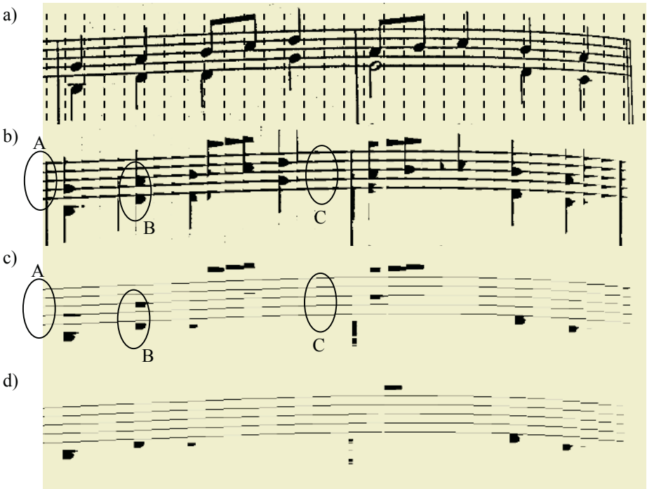
Fig. 2. Stages of histograms completing: part of original image (Fig. 1) sliced into vertical strips (a), local histograms H_i of horizontal projections (b), local histograms after pre-processing (c) and after final filtering (d)
