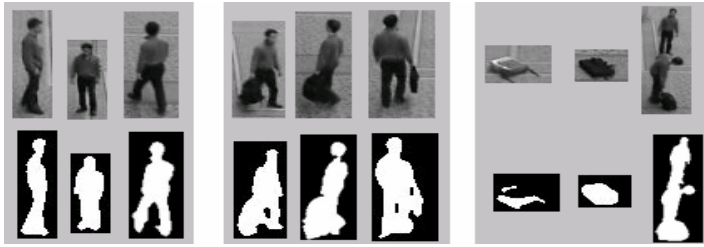
Fig. 3. Example grey-scale and binary images in three classes: a human without a bag, a human with a bag, and the unknown class
