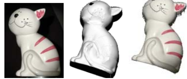
Fig. 8. Left: original image of porcelain cat with a small amount of paint added. Centre: recovered depth map. Right: mapping of original colours onto the surface.
