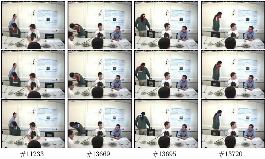
Fig. 2. Tracking using joint color-spatial distribution
