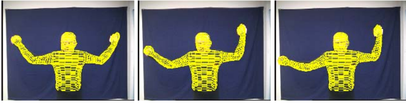
Fig. 9. Arms and head tracking of the “Reinhard”-model
