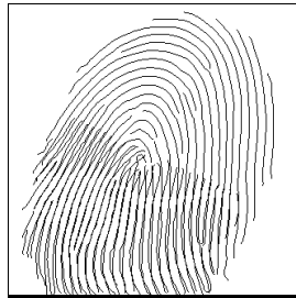
Fig. 2. In the reference ridge map, many ridges are broken due to the upper region of the fingerprint not being captured
