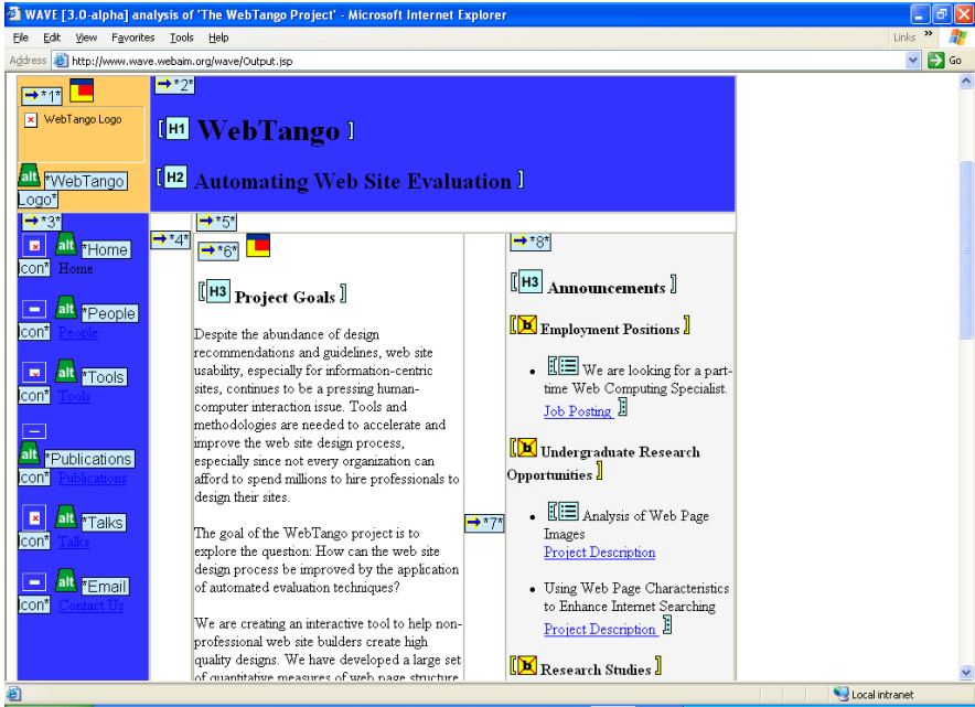
Fig. 1. Evaluation report produced by WAVE, where guideline violations are overlaid on the actual web page by using icons to flag potential issues and also depicts the page reading order (arrows with numbers)
