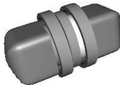
Fig. 6. A new version of the SquareBone: The manipulated handles are round allowing comfortable manipulation of diagonal movements. The square caps on the left and right side provide a tactile coordinate system.
