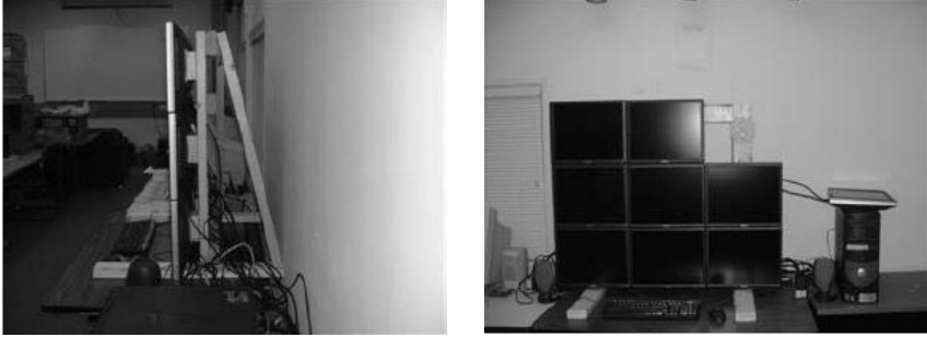
Fig. 3. The left figure shows the side view of the tiled display, showing how the monitors connect to the frame. The right figure shows the front view of the tiled display, with one monitor disconnected to show the underlying wooden frame. The sole computer powering the display is shown to the right.
