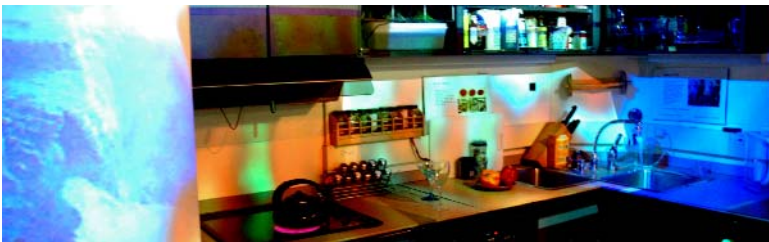
Fig. 1. Cooking with the Elements: Multimedia projections enrich a conventional kitchen by projecting intuitive displays to reveal the status of tools and surfaces
