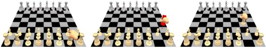
Fig. 2. User interaction using direct manipulation (virtual hand technique) with visual feedback. From left to right: picking , moving and dropping a chessman.
