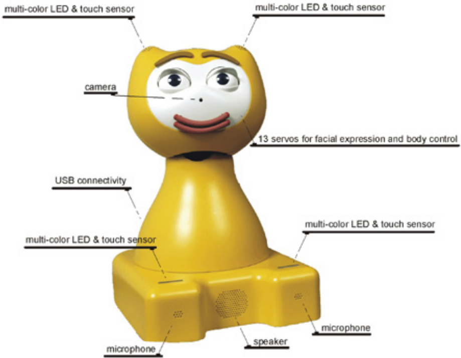
Fig. 1. Hardware setup of the home dialogue system “iCat”
