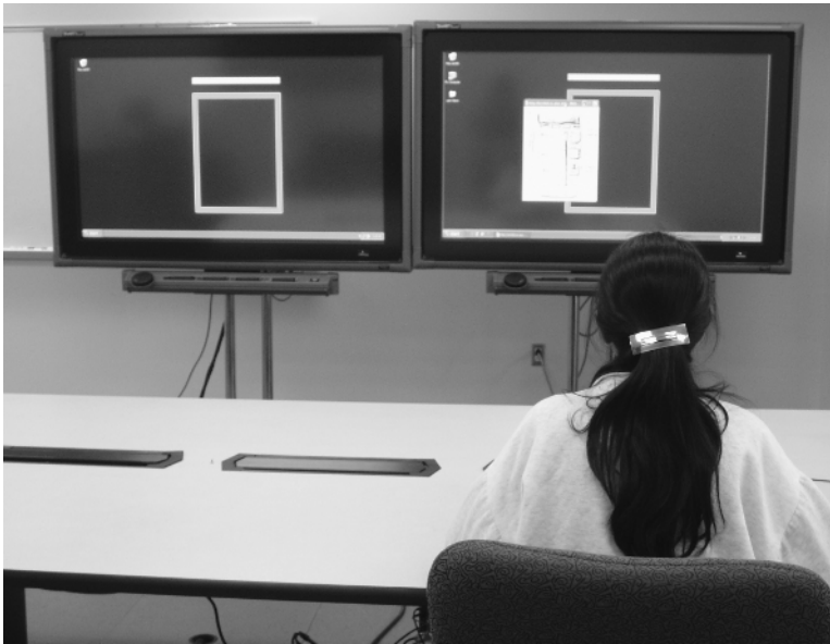
Fig. 2. A user is performing the experimental task for the 63" distance configuration. The user is moving an Internet Explorer application from the display on the right to the display on the left. After moving the application into the target box on the left, the user selects the rectangular bar above it. Each movement was a single trial and sixteen trials (resulting in a back and forth movement of the application) were performed in each configuration. The target boxes were used to ensure that the application was moved the same virtual distance.
