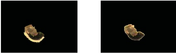
Fig. 8. Removing of shadow effect: (a) segmentation result with shadow effect; (b) segmentation result after a sobel operator applied
