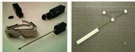
Fig. 2. Tracking and interaction devices. Left: Cameras, shutter glass and calibration stick, Right: Interaction stick
