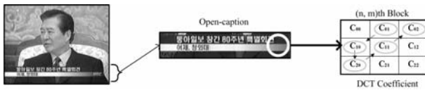
Fig. 4. Searching area for extraction and DCT coefficient
