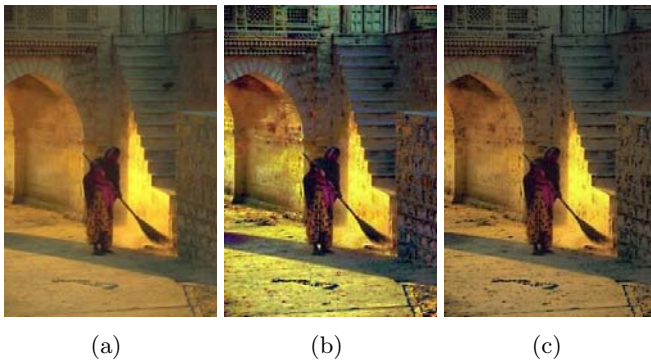
Fig. 5. (a) Original image, (b) algorithm from Sec. 2.2 applied with \delta = 2 on the red, green and blue channels separately. Note the significant hue shift towards purple in the stairs, arch and wall and towards green on the ledge above the stairs, (c) Using the method described in Sec.3 with \delta = 2 (separating the image into luminance and chrominance and applying the method to the former). Note that hue is preserved.
