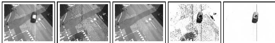
Fig. 3. From left to right: a frame in the middle of sequence S3; the corresponding backgrounds computed by alg. [3] and ours; the foreground pixels
