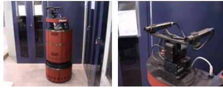
Fig. 1. Material used to develop the application. B21r Robot and Sony XC999 cameras.
