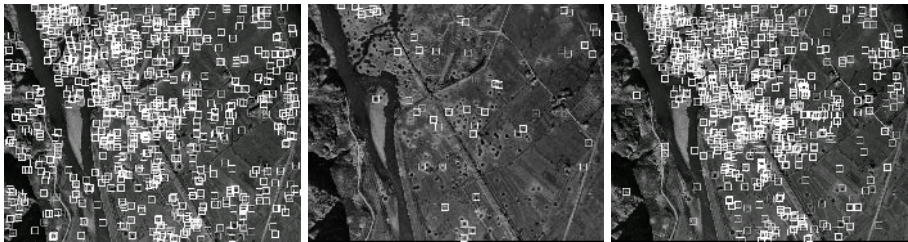
Fig. 4. The left image shows the classification obtained by applying SSTBoostReg, without spatial analysis. The middle image shows the “high margin craters” and the right image includes all the craters recognized by the local thresholding procedure.
