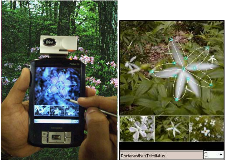
Fig. 2. M-CAVIAR graphic user interface. The model does not have to be perfect to rank the unknown in the top 3
