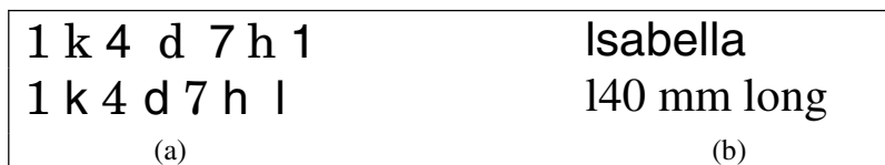
Fig. 4. (a) Style: in the part numbers on the left, the first pattern in the top row must be the letter l, and the identical first pattern in the bottom row must be the numeral 1. (b) Language context: here the surrounding text disambiguates the identical glyphs in either row.
