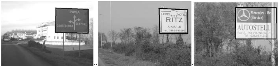
Fig. 4. Classification results indicated by the black frame: urban sign (left) and advertising (center), an advertising sign partially hidden by a pole (right).
