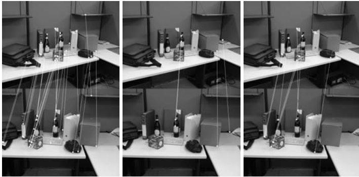
Fig. 2. Results for a 13-frames image sequence. Correct matches between first (top) and sixth (bottom) frame. Left: S-SVD. Centre: C-SVD. Right: S-DIST.
