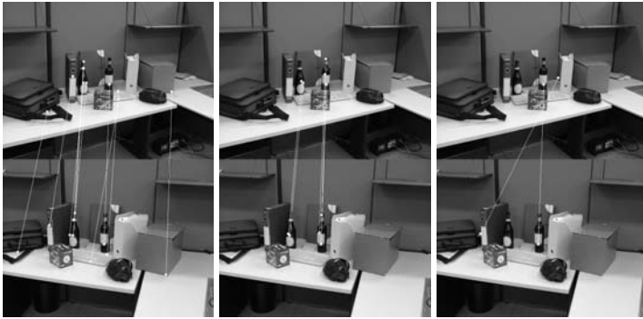
Fig. 3. Results for a 13-frames image sequence. Correct matches between first (top) and eightieth (bottom) frame. Left: S-SVD. Centre: C-SVD. Right: S-DIST. One of the matches in the right image is wrong but the two points lie on corresponding epipolar lines, therefore is wrongly passed as correct.
