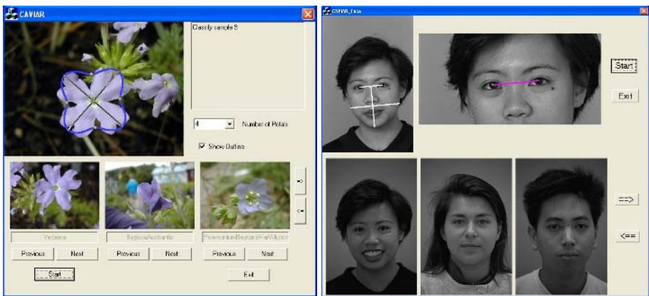
Fig. 1. CAVIAR-flower (left) and CAVIAR-face (right) visible models and graphic user interfaces. Because pupil localization is so important in face recognition, an enlarged view is provided for this part of the visible model.
