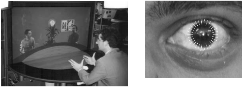
Fig. 1. Left: an immersive videoconferencing session. Right: active ellipse located around correct iris contour, and segments used to sample intensities.
