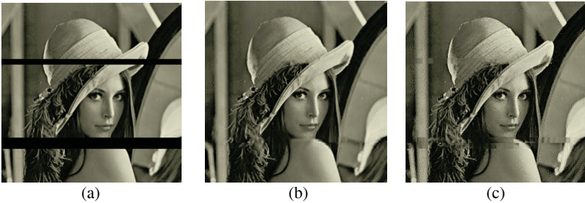
Fig. 5. The performance of different recovery methods; (a) the image damaged with losing three rows of blocks, (b) reconstructed result using the proposed method, (c) reconstructed result using Shao's method
