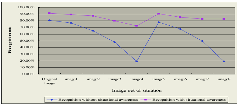
Fig. 6. Comparison of recognition rates using fixed Gabor representation and that using adaptive Gabor representation for each illumination situation
