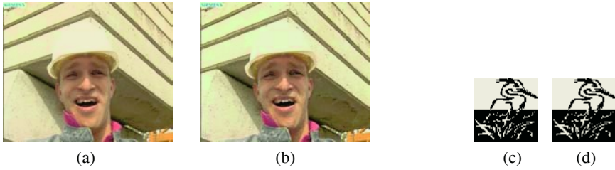
Fig. 2. Simulation results of foreman sequence. (a) Original 30 th frame; (b) Watermarked 30 th frame when QP=4 ; (c) Original watermark; (d) Extracted watermark
