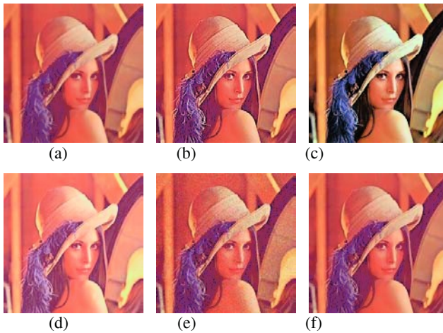
Fig. 4. (a) More blurring. (b) More sharpening. (c) Histogram. (d) Brightness adjustment (+40). (e) Gaussian noise( \sigma = 20 ). (f) JPEG compression(30%).
