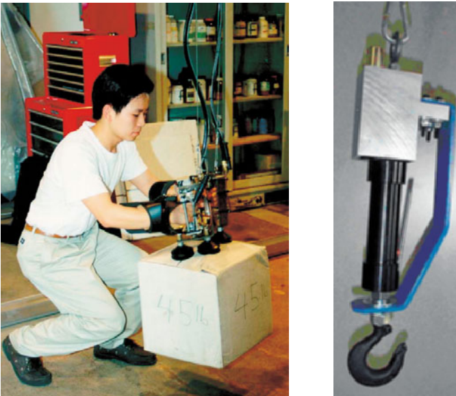
Figure 3: Intelligent Assist Devices (IAD): the simplest form of upper extremity enhancers for industrial applications
