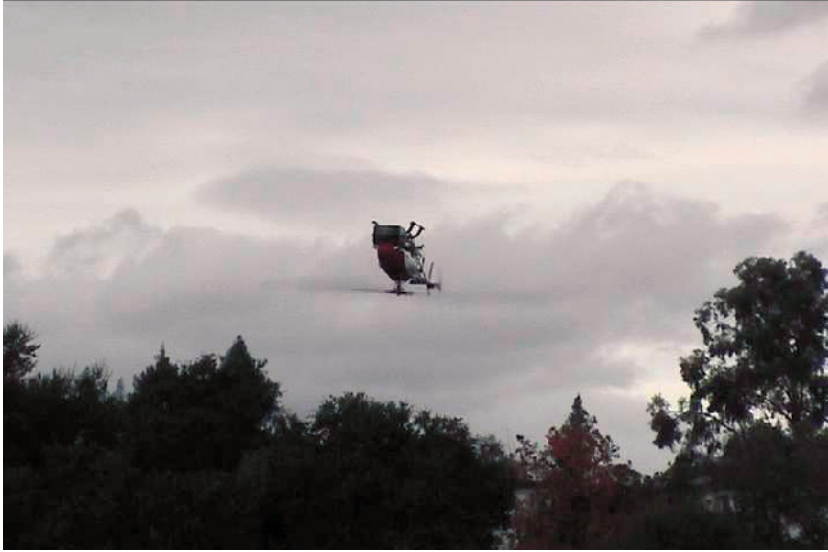
Fig. 3. Helicopter in autonomous sustained inverted hover.
