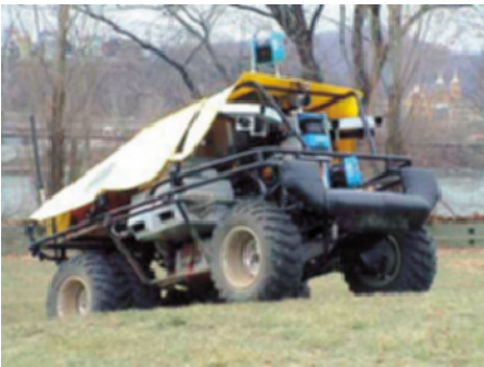
Fig 1: Autonomous Ground and Air Vehicles. A Honda ATV and Yamaha Rmax Helicopter were retrofitted for autonomy.
