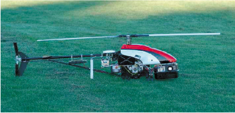
Fig. 1. Helicopter in configuration for upright-only flight (single GPS antenna).
