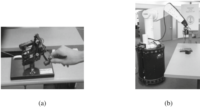
Fig. 5. System Setup. (a) Phantom TM device controlled by a human. (b) PUMA robot mounted on XR4000 (ROME0)
