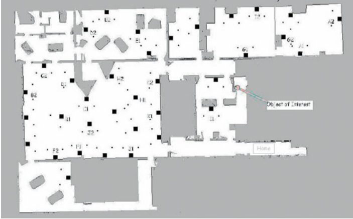
Fig. 6. Autonomously planned sensor net positions (black squares) and planned leader waypoints associated with each sensor position (small dots).
