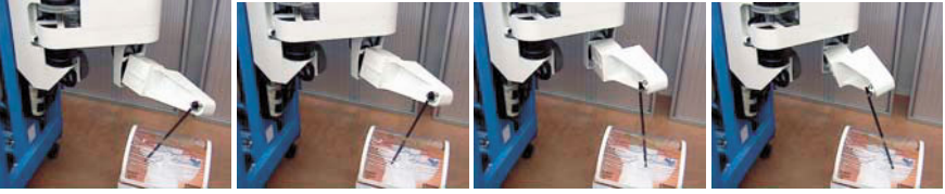
Fig. 4. Straight line motion of D2M2 under constraint of trocar.
