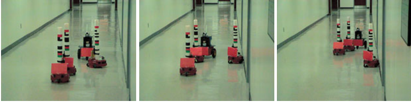
Fig. 5. Deployment of a sensor robot using assistive navigation: the lead robot first guides and then directs the sensor robot into position.
