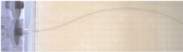
Fig. 4. (Top) The nonholonomic model fit to the average double bend experimental needle path. (Bottom) During the experiment, the needle was inserted 8.3 cm, spun 180°, then inserted another 16.7 cm.
