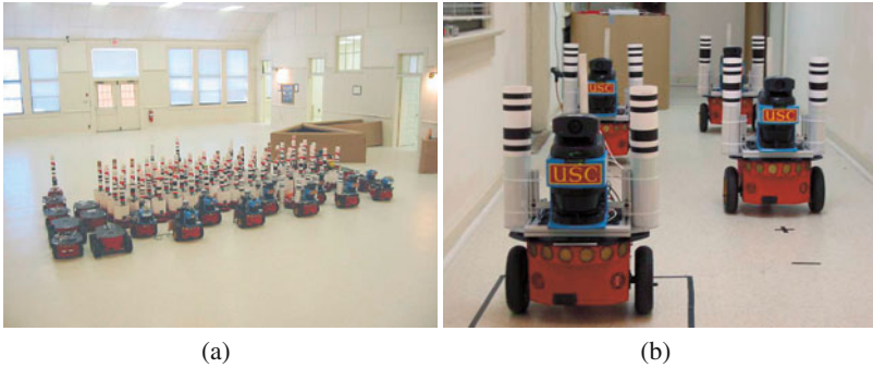
Fig. 1. (a) The heterogeneous robot team, with three classes of robots (mapper, leader and sensor); the sensor robots are based on the ActivMedia AmigoBot. (b) The mapping sub-team: note each of the four robots carries a unique laser-visual fiducial; these fiducials can be detected and identified at ranges in excess of 8m, and the relative range and bearing of the robots can be determined to within a few centimeters and a few degrees, respectively.
