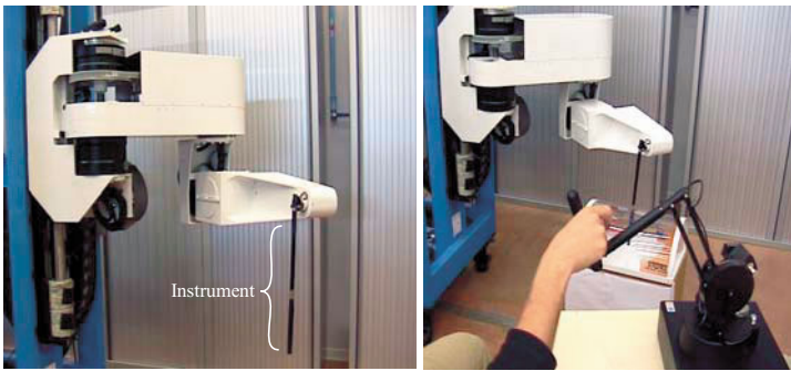
Fig. 2. The 5-dof robot D2M2 and the Phantom master device.
