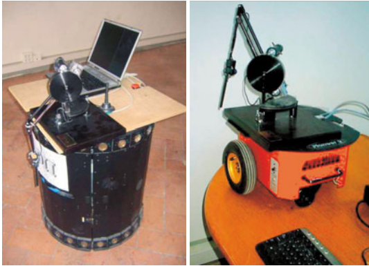
Fig. 1. Two mobile haptic interfaces: a general purpose interface based on the holonomic Nomad mobile robot and a Phantom Premium 1.5; a more limited interface based on a non-holonomic Pioneer mobile robot and a Phantom Premium 1.5
