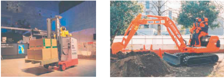
Fig. 3. Teleoperated humanoid drives a lift truck (left) and a backhoe (right)
