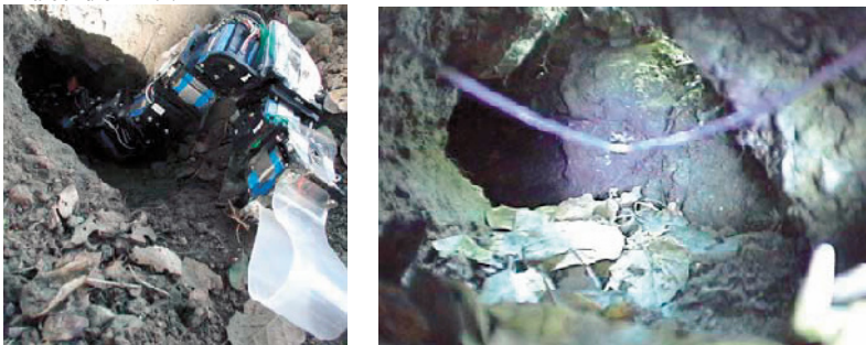
Fig. 8: a) Concertina gait moving through ground squirrel hole. b) Inside of the hole as seen by robot's camera
