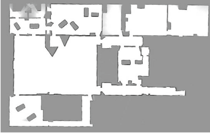
Fig. 4. Occupancy grid map produced during a multiple-robot, multiple-entry trial: two robots entered from the door at the right top, another two robots entered from the door at the right bottom (the relative pose of the two doorways was unknown). The environment is approximately 45 by 25 meters in size, with an internal area of 600 m 2 .
