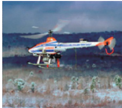
Fig 1: Autonomous Ground and Air Vehicles. A Honda ATV and Yamaha Rmax Helicopter were retrofitted for autonomy.
