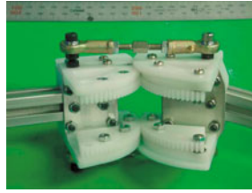
Fig. 5. two-axis rolling contact joint of knee; distance of the two axes is fixed and the gear surface avoids slipping.
