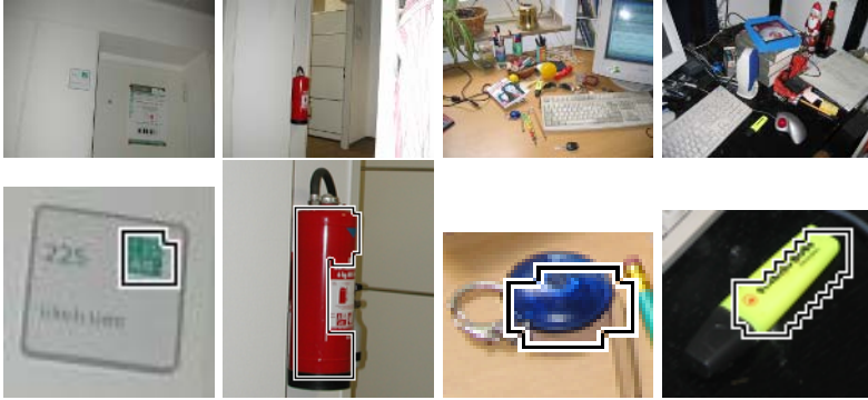
Fig. 3. Top: the training images with the targets (name plate, fire extinguisher, key fob, and a highlighter on the dark desk). Bottom: The part of the image that was marked for learning (region of interest (ROI)) and the contour of the region that was extracted for learning (most salient region (MSR)).
