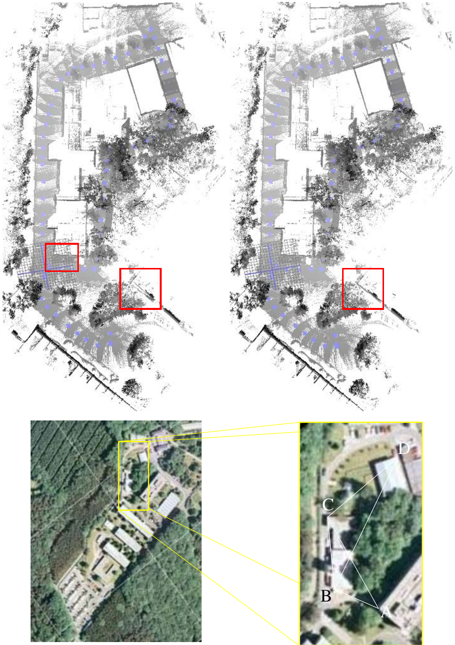
Fig. 4. Top left: Model with loop closing, but without global relaxation. Differences to Fig. 3 right and to the right image are marked. Top right: Final model of 77 scans with loop closing and global relaxation. Bottom: Aerial view of the scene. The points A – D are used as reference points in the comparison in Table 1.
