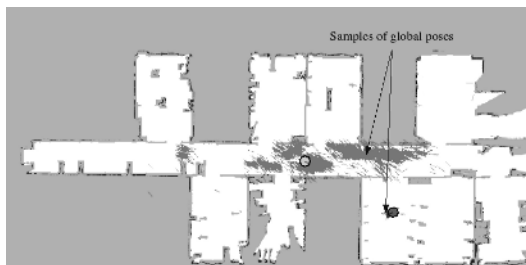
Fig. 5. Dark robot drives into an office and localizes itself globally
