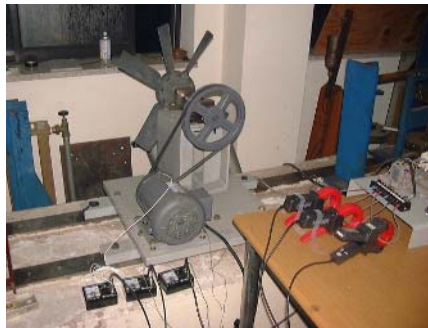
Fig. 3. Fault detection and data acquisition equipment
