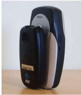
Fig. 2. An Active Bat attached to a Bluetooth capable mobile phone used to correlate signal strength readings with their locations
