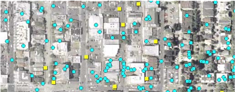
Fig. 2. An overhead satellite map showing the results of self-mapping using the hotspot finder seed set. The squares mark the locations of the beacons in the seed set, while the circles denote the beacons placed by the self-mapping algorithm
