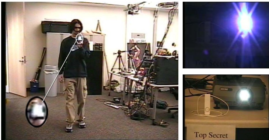
Figure 5. Left is a camera phone being neutralized by our system (notice the neutralizing light beam over the lens). Top right is the camera view neutralized by the system and bottom right is the camera view when the camera is permitted to capture.
