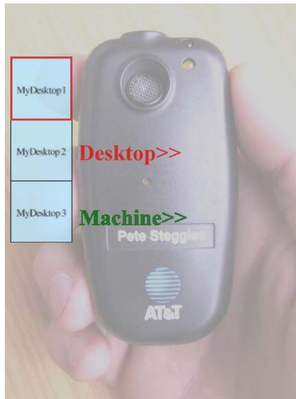
Fig. 5. The augmented view of a Bat while inside a teleport region. Square menu items show desktop names (here too, the composite picture is simulated).
