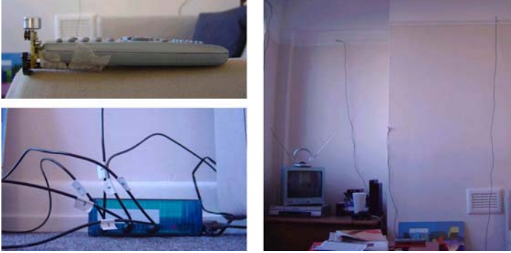
Fig. 9. An initial deployment of the ultrasonic tracker within the home. Tag attached to a remote control (top left). Ultrasonic controller (bottom left) and receivers attached to walls (right).
