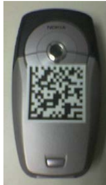
Figure 6. A 5 cm x 5 cm retro-reflective glyph pattern is temporarily attached near a camera phone’s lens.
