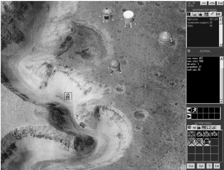
Fig. 1. Gray-scale snapshot of the simulator. On the planetary surface, from top to bottom: A cargo, a habitat, a greenhouse, a nuclear reactor, an astronaut driving a light vehicle (selected), an astronaut walking and another light vehicle. The right panel is divided into 3 parts. At the top, information on the selected object is available. A journal provides information on current events (action completed, oxygen missing, etc.). In the middle, a small grid enables the selection of astronauts and at the bottom, transformations icons are displayed in different grids.
