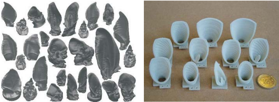
Fig. 1. Pinna shapes: (a) Scanned bat pinnae (micro-CT), (b) Nylon pinnae (selective laser sintering)
