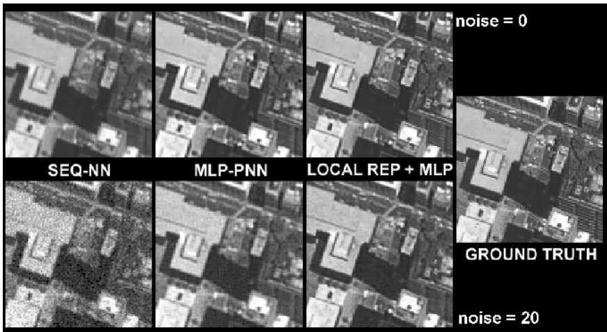
Fig. 3. Superresolution results, for a scaling factor of 2, on a synthetic sequence of an urban area using different methods. In the first row, are presented the results for a noiseless input sequence. The second row contains the results for a sequence corrupted with Gaussian noise of \sigma = 20 gray levels. Each column contains the results of a different method. The ground truth is presented at the right of the image.
