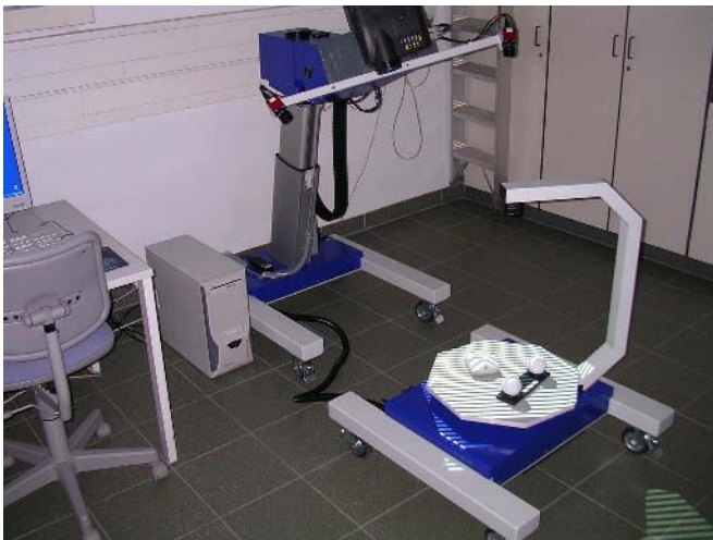
Fig. 1. 3D measuring system “kolibri-flex” using fringe projection
