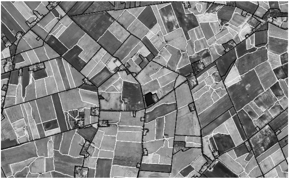
Fig. 2. Exemplarily result of the segmentation: black lines are the borders of the regions of interest generated from the GIS-data, white lines are the preliminary field boundaries
