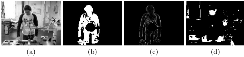
Fig. 1. Information used for tracking: (a) Input image (b) Foreground map (c) Gradient information (here vertical edges) (d) Skin-color map
