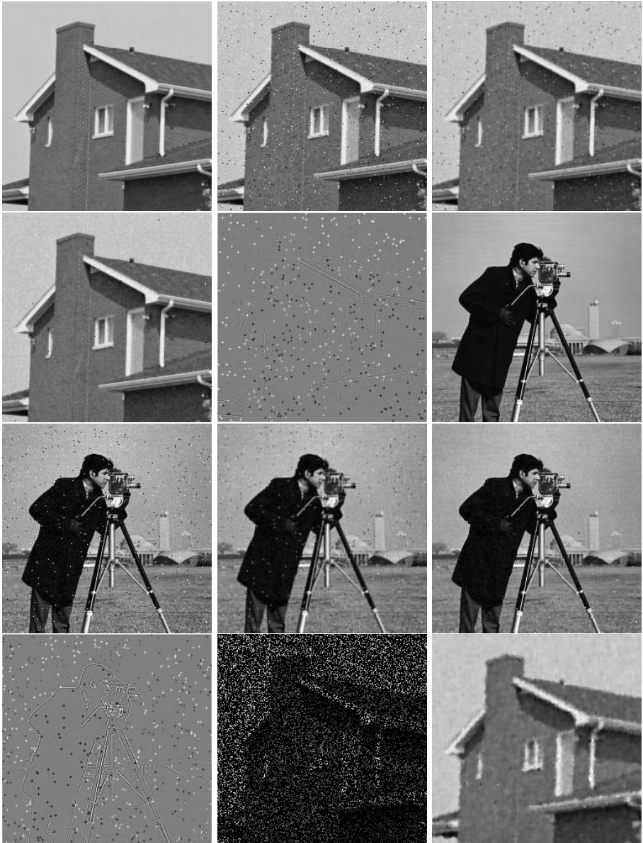
Fig. 2. Denoising experiment. Row-wise from top left to bottom right: House image: original, noisy ( \sigma = 10^{-3} , 1% Salt & Pepper noise), Wiener filtered, Wiener channel smoothed, difference between linear wiener filtering and Wiener channel smoothing (amplified by factor two); cameraman image: original, noisy ( \sigma = 10^{-3} , 1% Salt & Pepper noise), Wiener filtered, Wiener channel smoothed, difference between linear wiener filtering and Wiener channel smoothing (amplified by factor two); randomly sampled house image image (25% samples, \sigma = 10^{-3} ), inpainting result from normalized averaging.
