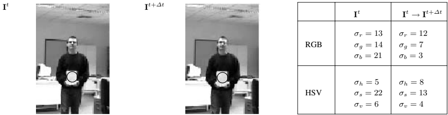
Fig. 1. Example showing the change of color over time because of independent changes of brightness and contrast within different color channels. The color components of an image pixel can change over time because of reflection and illumination changes.
