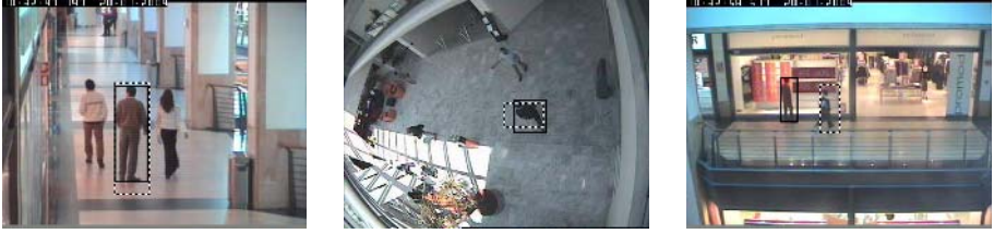
Fig. 2. Stills from three of the videos used. The solid box marks the hand-labeled ground truth. The dashed box is the tracker’s current estimate. In the right-most image, the tracker has been distracted by a temporary occlusion from another person, and subsequently lost the real target.
