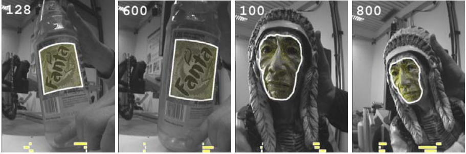
Fig. 2. Screenshots of the tracked sequences bottle and sculpture . The region of the tracked 3-D model points is manually outlined for better visualization.
