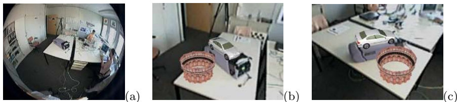
Fig. 5. (a) Original fisheye image, (b) and (c) video augmentation of a perspective cutout of the fisheye sequence from different view points
