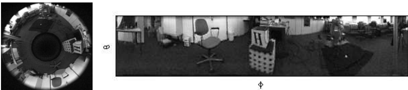
Fig. 4. Image captured with a parabolical mirror and its mapping to V(\phi, \theta)
