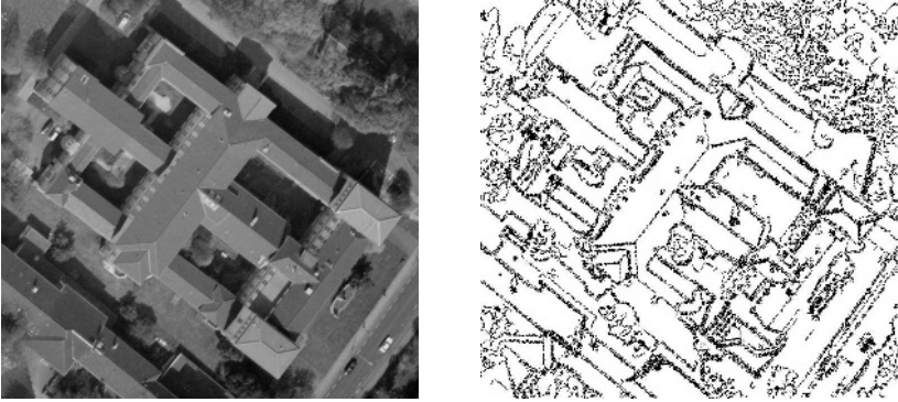
Fig. 1. 1000 \times 1000 pixel patch cut out of an aerial image and the extracted edgels
