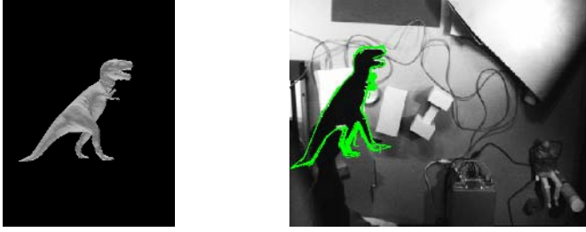
Fig. 1. One of the generated training images (left) and the recognition result (right) for a free-form object. It was sufficient for this object to learn and represent the silhouette.
