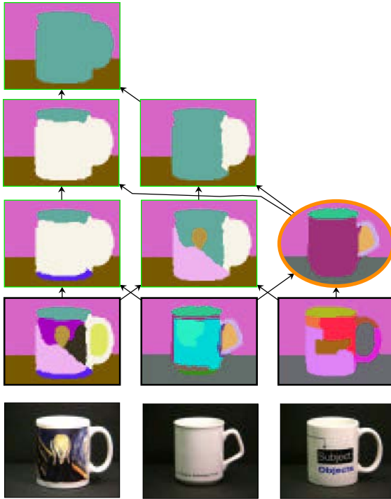
Fig. 4. Computed LCA (orange border) of 3 examples. From a set of three region adjacency graphs representing the appearance of three different cup exemplars, the algorithm extracts the salient surfaces of the cup, including the body, inside surface (ellipse at top), handle, and hole (indistinguishable from a real surface). Figure taken from [3], copyright IEEE, 2005.
