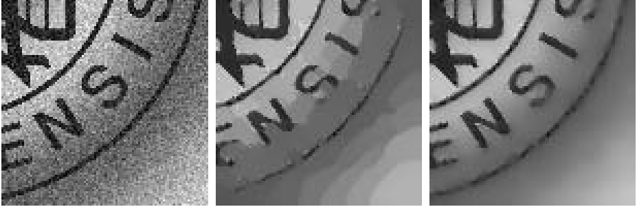
Fig. 1. (a.) Left: Initial noisy image. (b.) Middle: Second order Perona-Malik filtering. (c.) Right: Linear combination of second and fourth order Perona-Malik filtering.
