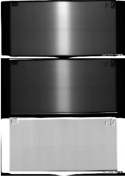
Fig. 3. Acrylic Test Phantom - Top: Background Image; Middle: Diagnostic Image; Bottom: Reconstruction Image (enhanced for a better detail view).
