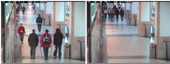
Fig. 2. Tracking result for one of the images sequences from the CAVIAR test bed (first and last image of the successfully tracked person). Ground truth and computed region of the moving person (ellipses) are almost the same, even in the case of change in scale.
