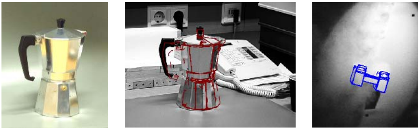
Fig. 4. Real training image (left) and recognition result (middle) for a highly specular object. Detected barbell (right) under extensive occlusion by fog.
