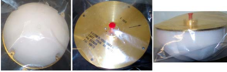
Fig. 6. Three images of a flight antenna; the evolved wire configuration for the radiator sits on top of a 6" diameter ground plane and is encased inside a radome.
