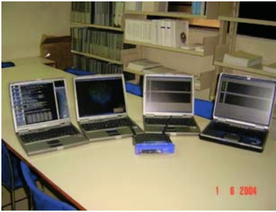
Fig. 5. (Left) Minicluster mobile wireless/fast-ethernet, (Right) Performance comparison between wireless and fast-ethernet networks
