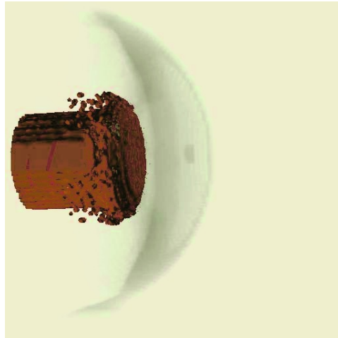
Fig. 3. 3D simulation of diesel injection with 2.5 million particles. The picture shows the injected diesel. First drops are already split off the jet. The injection causes a density wave traveling in front of the liquid stream.
