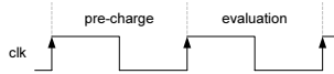
Fig. 10. Sequence of pre-charge and evaluation phases in an MDPL circuit using MDPL D-flip-flops without timing constraints
