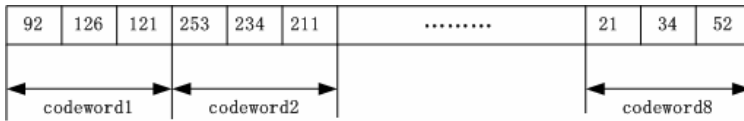
Fig. 3. This figure shows the encoded string of a particle for an eight-length in a three-dimension
