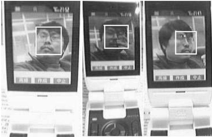
Fig. 6. Sample experiment results of our mobile phone embedded face detection system on real-time detection
