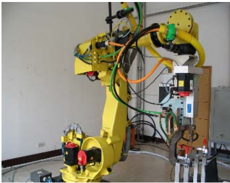
Fig. 1. Experimental system using servo gun
