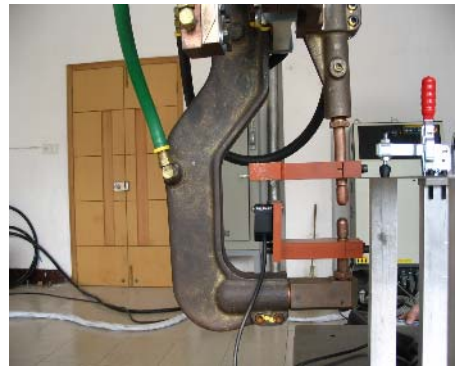
Fig. 2. Fixture for installing sensor
