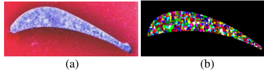
Fig. 4. The section of blade added chemical refiner: (a) Optical micrograph and (b) simulated grain structure
