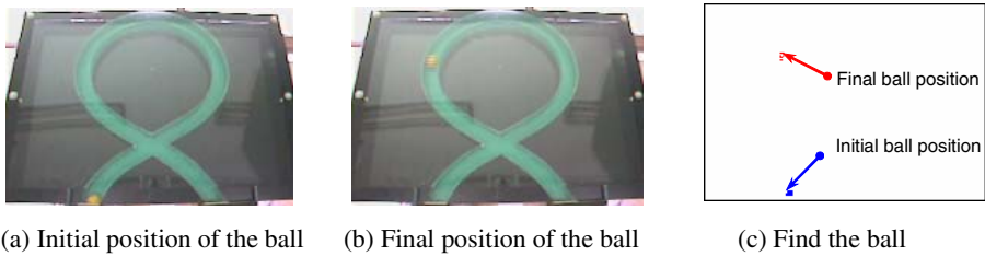
Fig. 2. Image processing to determine the ball position
