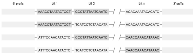
Fig. 1. Examples of possible words of n -bits. Each bit can consist of 15 nucleotides. Furthermore, each bit is unique and should not hybridize to other bits nor to itself.
