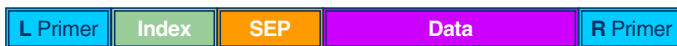
Fig. 2. A DNA database element with a separation element (SEP) between the index and data parts. Double border rectangles represent double stranded sequences.
