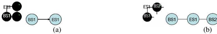
Fig. 1. (a) Example of directed edge. ES1 is surrounded by BS (b) Example of undirected edge. ES1 is adjacent to BS1 and BS2.
