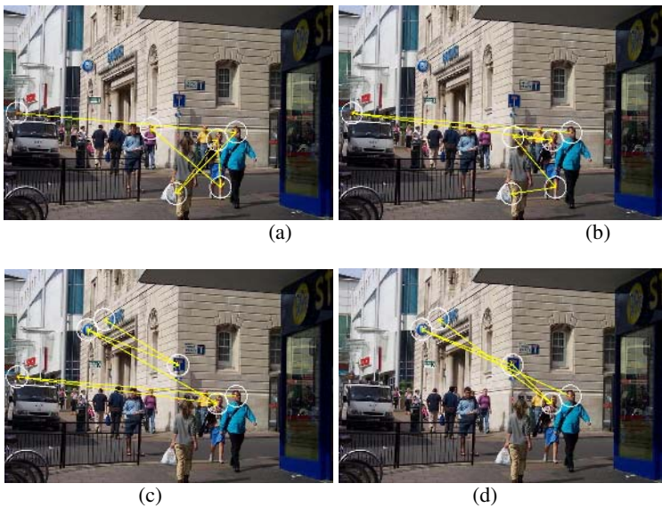
Fig. 4. The attention trajectories varied by different values of \alpha and \beta . The task for the model is to find the person who is wearing blue color t-shirts. (a) \alpha=1.0 , \beta=0.0 (b) \alpha=0.6 , \beta=0.4 (c) \alpha=0.5 , \beta=0.5 (d) \alpha=0.4 , \beta=0.6 . Even a small amount of \beta is enough to change the trajectory of attention. Adding more to \beta produced a strong tendency that the trajectories of attention are attracted closely to the location of a cue color (blue) region.
