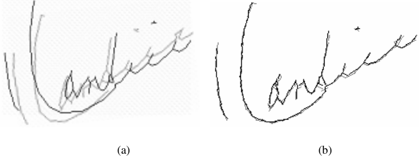
Fig. 4. (a) Overlapped image of the approximated skeletons of signature Template (black) and signature Input (grey) after global registration. (b) Overlapped images after elastic local alignment by deforming the Template .
