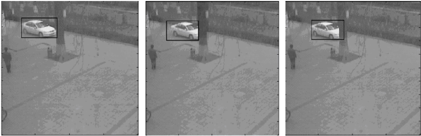
Fig. 2. Comparing our algorithm with the integral-intensity-matching algorithm. The first image: Tracking before occlusion, and both of the two algorithms can track accurately. The second image: the target is occluded locally, and tracking is false using the integral-intensity-matching algorithm only. The third image: Accurate tracking using the proposed algorithm in this paper (overcoming the local abruptly varying intensity problem).
