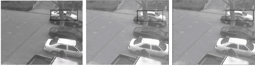
Fig. 4. The abruptly varying illumination handling. The first image: The correct tracking under occlusion before the illumination changes (the luminance is very dim). The second image: The illumination abruptly changes and tracking is false before we adopt the proposed solving method. The third image: The correct tracking using our proposed method.
