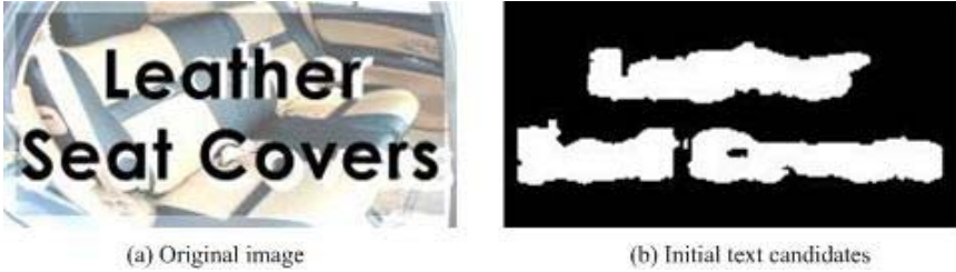
Fig. 2. Initial text candidates: (a) is original image, and (b) is the result of initial text candidates after classification
