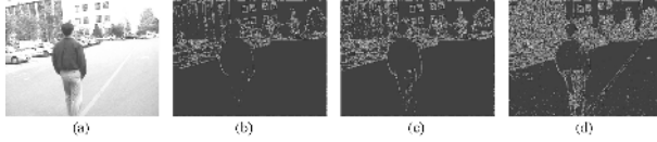
Fig. 3. Multi-level canny edge, (a) an input frame (b) the 1st level edge (c) the 2nd level edge (d) the 3rd level edge
