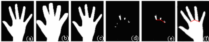
Fig. 1. Get the triangle regions from binarized source hand image, (a) Binarized hand image, (b) Dilated, (c) Eroded, (d) Triangle regions, (e) Connect the key points, (f) Rotated
