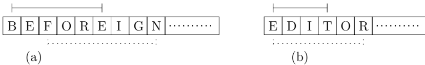
Fig. 1. The figure illustrates the leftmost non-overlapping match rule. (a) When the pattern is {BEFORE, FOREIGN}; the rule chooses BEFORE. (b) When the pattern is {EDIT, EDITOR}; the rule chooses EDIT.
