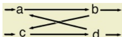
Fig. 3. If ab and cd are DAG edges, then the two non-DAG edges da and bc are mutually exclusive, since using them both leads to the wrong order for a and b .
