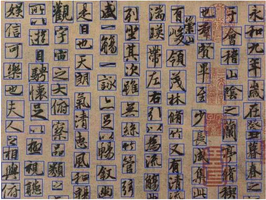
Fig. 2. An example of segmenting a page into individual characters using minimum-bounding box
