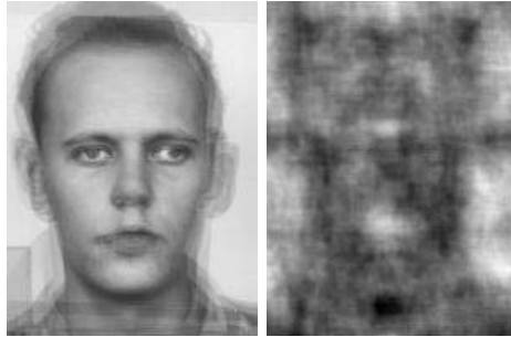
Fig. 2. Sample images for an implementation of the biometric encryption technique of [14] applied for a face recognition. Left: Image f_0 averaged from five samples. Right: Template h_0 including the random phase encoded elements
