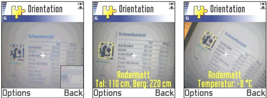
Fig. 2. Selection from a table: the code coordinates determine the table row, the camera rotation specifies the concrete information aspect to display
