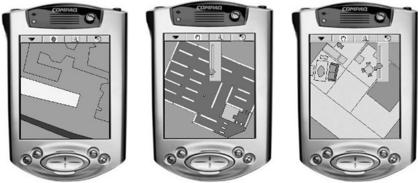
Fig. 1. Example screenshots of the simple map-application with different maps. The toolbar on top allows easy access to scrolling mode, as well as zooming and rotating the map
