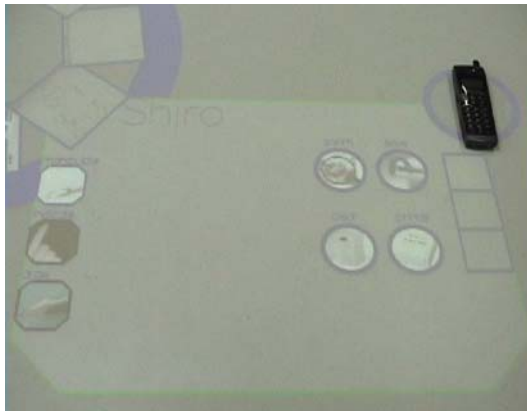
Fig. 4. A private workspace. The mobile phone, the top-right position in this example, defines a reference point. The three icons on the left are operational icons. The four icons on the right are data icons
