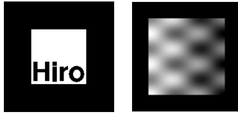
Fig. 1. A sample template from the ARToolKit distribution (left) and from the maximum distance set (right)
