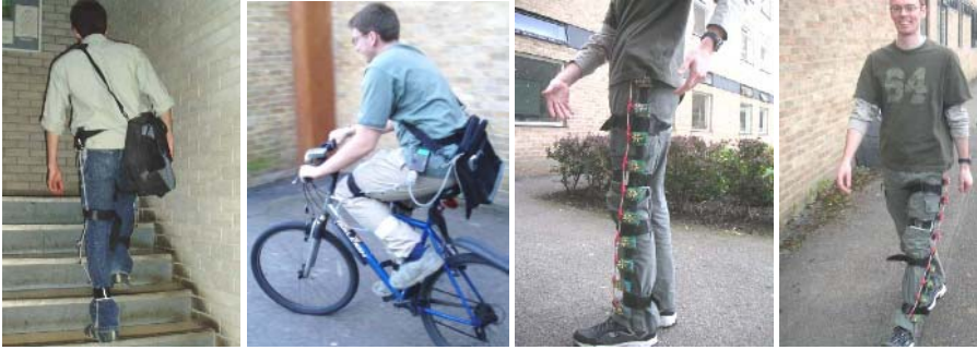
Fig. 6. Experiments of [10] with networks containing a large amount of motion sensors: the left two using 40 accelerometers, the right two using 90 tilt switches
