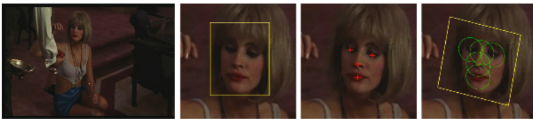
Fig. 5. (a) Original frame. (b) Close-up with face detection superimposed. (c) Detected facial features (eyes, nose, mouth). (d) Face is represented as a collection of local affinely deformed spatial orientation fields (SIFT descriptors). The green circles illustrate the location and support region for each of the five SIFT descriptors. Note how the position of the local regions adapts to the slightly rotated pose of the head in this case
