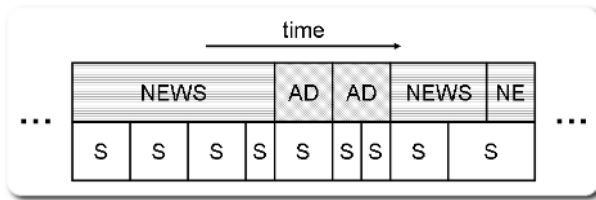
Fig. 1. The top row of the figure illustrates the boundaries between news stories and advertisements. The bottom row depicts the visual shot boundaries. Each story contains one or more shots. Story boundaries and shot boundaries need not align
