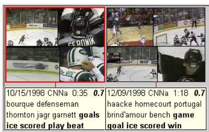
Fig. 5. Tooltips showing relevant keywords for the top two results pictured in Figure 4 for the query terms: “hockey”, “ice”. Words shown in bold are those closest to the query terms. Words in plain font are those with the highest tf*idf values. Note that the obvious query term, “hockey”, does not appear
