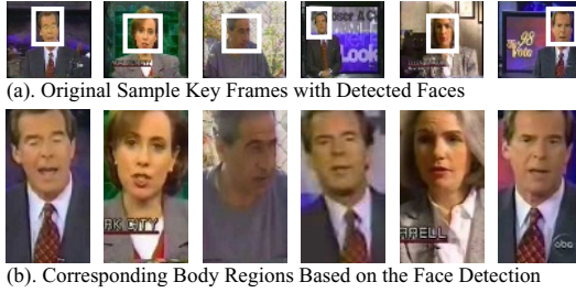
Fig. 2. (a). The sample key-frames with the detected faces; (b). The body regions extended from the faces. Global feature comparison or face correlation fails to cluster the same anchor together
