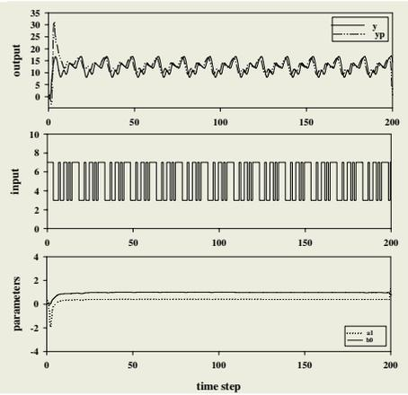
**Fig. 7.** DRLS identification with Model 1 and PRBS input
