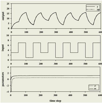
**Fig. 6.** DRLS identification with Model 1 and ternary input
