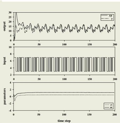
**Fig. 9.** CRLS identification with Model 1 and PRBS input
