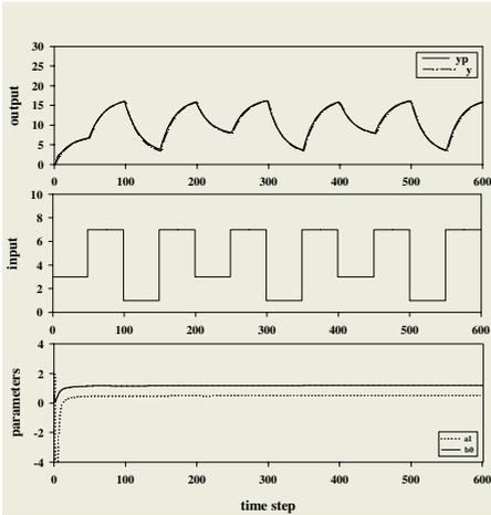
**Fig. 8.** CRLS identification with Model 1 and ternary input
