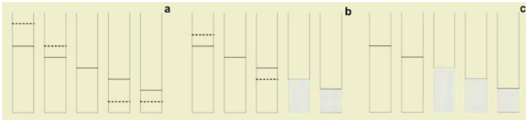
Fig. 1. A dashed (or solid) line indicates the Nash (or Optimum) load n_i (or o_i ) assigned to each machine i = 1, \dots, 5 . (a) Machines 1 and 2 (4 and 5) are over(under)-loaded while 3 is optimum-loaded. Then OpTop will assign load o_4 and o_5 to machines 4 and 5. (b) Now machines 4 and 5 received load o_4 and o_5 by OpTop . In the induced Nash assignment, machines 1 (3) become over(under)-loaded while 2 becomes optimum-loaded. (c) Finally, OpTop assigns load o_3 to machine 2. In the induced Nash assignment, machines 1 and 2 become optimum-loaded
