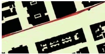
Fig. 7. The trace of Figure 6, fitted to a line drawn along the kerbside using the GPS correction tool
