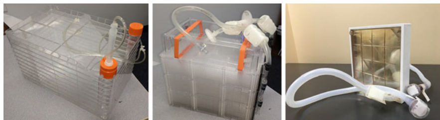
Fig. 1 2D platforms; Nunc ® 10 layer Cell Factory ( left ), Corning ® 32 layer Hyperstack ® ( center ) and CellCube ® ( right )
