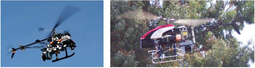
Fig. 1. Instrumented helicopter platform: The system is based on the Bergen Industrial Twin, with a modified SICK LMS laser range finder, a Crossbow IMU, a Honeywell 3-D compass, a Garmin GPS, and a Nikon camera. The system is equipped with onboard data collection and processing capabilities and a wireless digital link to the ground station.
