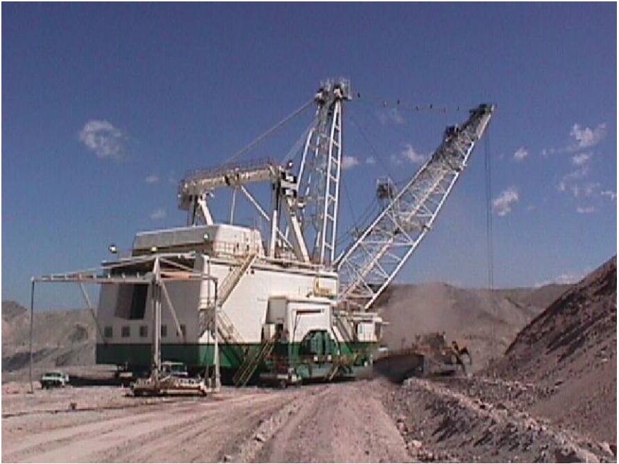
Fig. 1. The Bucyrus-Erie 1350 dragline at Boundary Hill mine, Queensland, which was used for our testing. The boom is 100m long.
