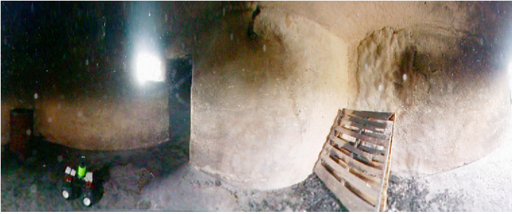
Fig. 8. 360 degree panorama of a room in the burning building taken by a catadioptric system. The image can be viewed using a combination of a head tracker/head mounted display to enable a digital pan and tilt with very low latency.
