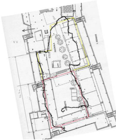
Fig.3. Human dead reckoning with DRM and IMU. Walked distance is about 200m and the real route was enclosed.
