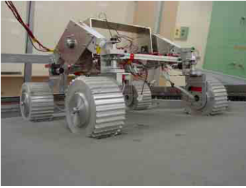
Fig. 6. A setup for slope climbing experiments by a 4-wheel drive rover test bed on Regolith Simulant
