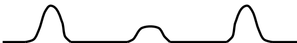
Fig. 7. A potential field which is more intuitive to the driver than the one in Figure 6. Flat sections in the middle of each lane where there is no interference with the driver's intention and it is more difficult to departure from the road than to cross lanes.
