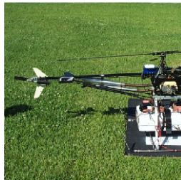
Fig. 1. AVATAR ( Autonomous Vehicle Aerial Tracking And Reconnaissance) after landing on a stationary helipad
