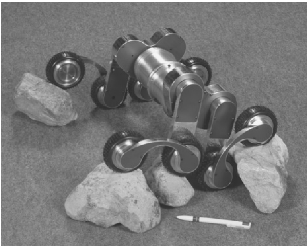
Fig. 5. Octopus features an active locomotion concept with 8 motorized and tactile wheels, 6 active and 1 passive DOF for ground adaptation and on-board integration of all control elements, joint sensors and inclinometers. (Photo © Bramaz)
