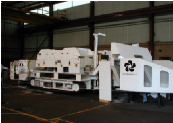
Fig. 1. The ACBM showing tramming platform, automatic bolting rigs, receiving hopper, bolt storage and delivery system.
