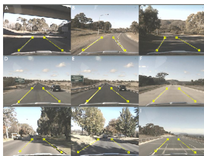
Fig. 4. Results from the lane tracker. The boxes indicate the end of the lines that mark the tracked lane.
