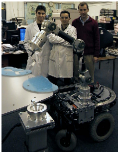
(a) Robot attached to the wheelchair with the spoon tool-holder
