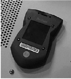
Fig. 2. A radio tag, approximately 12 × 9 cm in size, with which a robot can communicate to obtain range data. Such tags can be scattered into a burning building as firefighters move about or even be deployed by robots themselves. Since these tags are placed without careful survey, their position must be calculated along with the position of the mobile agents themselves.
