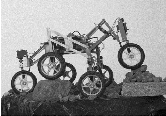
Fig. 4. The robot Shrimp is an all-terrain rover based on a passive locomotion concept. It is characterized by 6 wheels suspended by parallel mechanisms, one fixed wheel in the rear, two boogies on each side and one front wheel with spring suspension. The robot sizes around 60 cm in length and 20 cm in height, is highly stable in rough terrain and overcomes obstacles up to 2 times its wheel diameter with a minimal friction coefficient.
