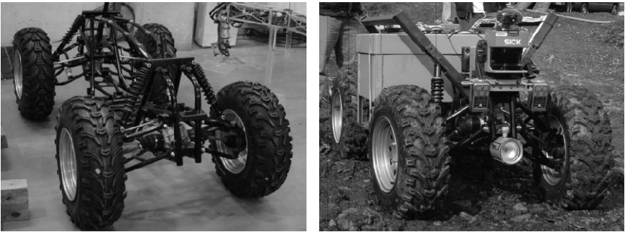
Fig. 1. Left: The base chassis, composed of two connected ATV front-ends. Right: Groundhog , 43 days later, just before its first deployment into an abandoned mine.
