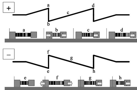
Fig. 4. Driving principle of XZ-stage
