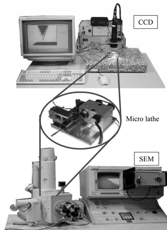
Fig. 1. Concept of the developed micro lathe
