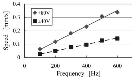
Fig. 5. Velocity change depending on frequency and voltage
