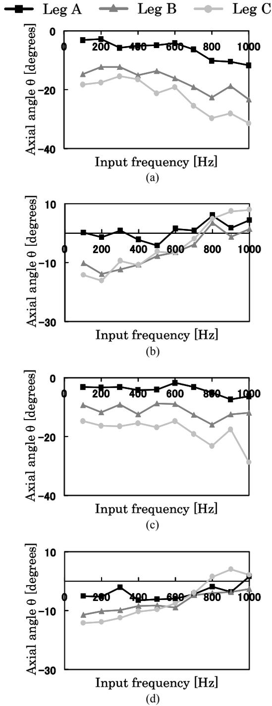
**Fig. 10**  $\theta$  of the legs of each frequency. (a) The control waveform is rectangle, and the direction is the CCW direction. (b) The control waveform is rectangle, and the direction is the CW direction. (c) The control waveform is sinusoidal, and the direction is the CCW direction. (d) The control waveform is sinusoidal, and the direction is the CW direction.
