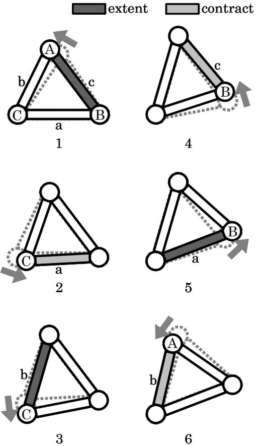
**Fig. 3** The motion mechanism in the CCW direction.
