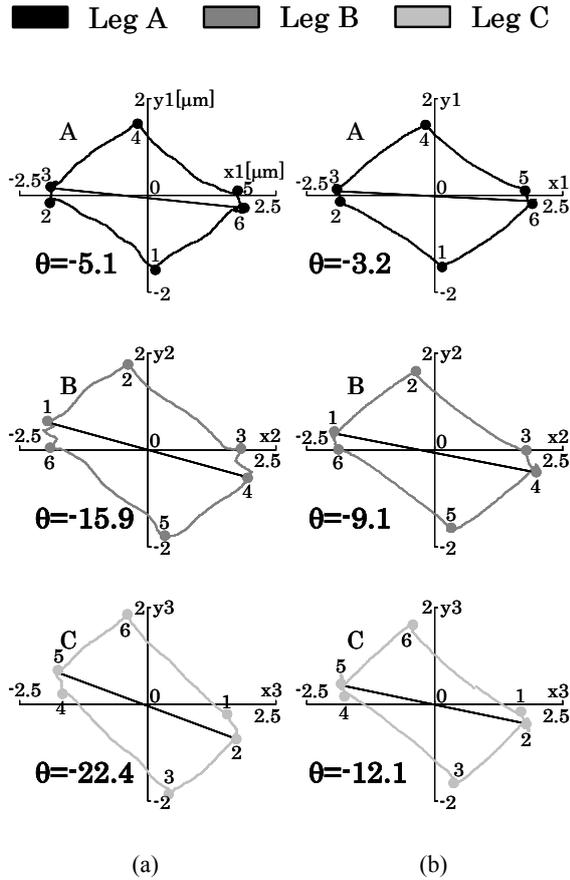
**Fig. 8** Three legs' trajectories in the local xy plane and the long axis angle  $\theta$ . The control waveform is rectangle. The direction is the CCW direction. The frequency is (a) 800 Hz and (b) 300 Hz.
