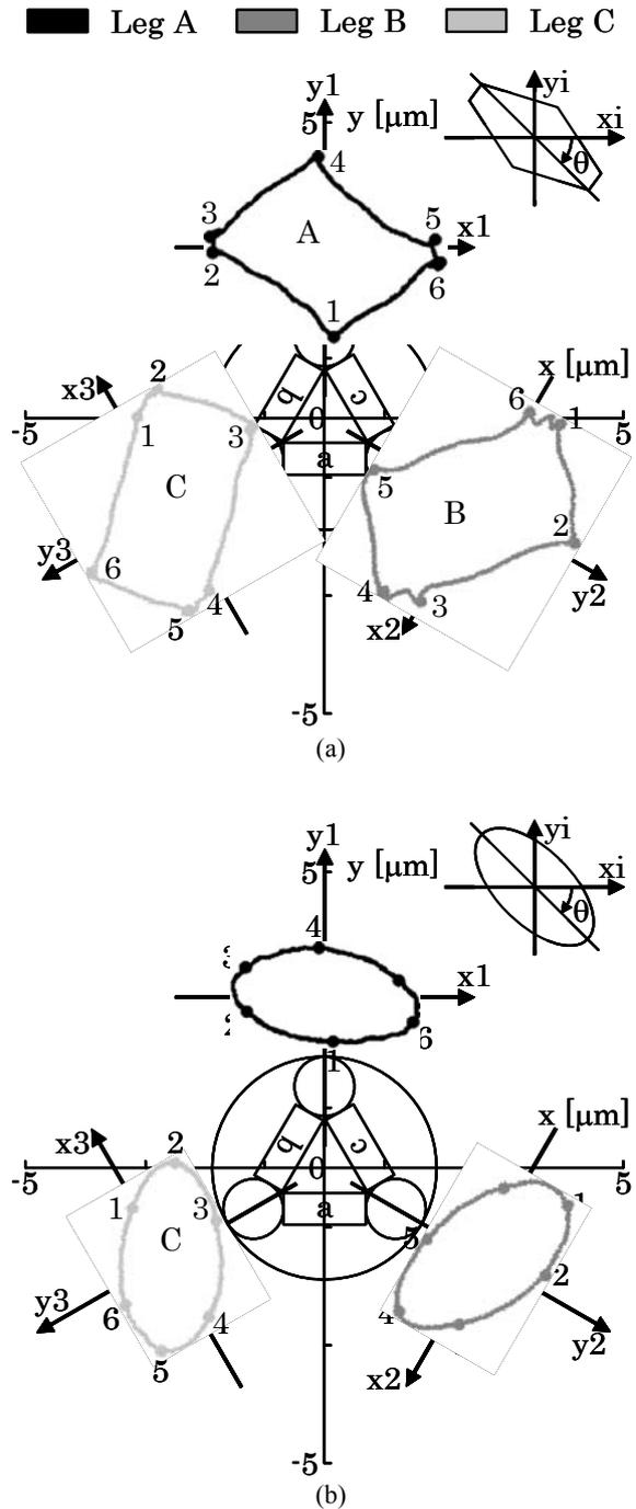
**Fig. 7** Three legs' trajectories in the local  $xy$  plane and the long axis angle  $\theta$ . The frequency is 800 Hz. The direction is the CCW direction. (a) The control waveform is rectangle. (b) The control waveform is sinusoidal.
