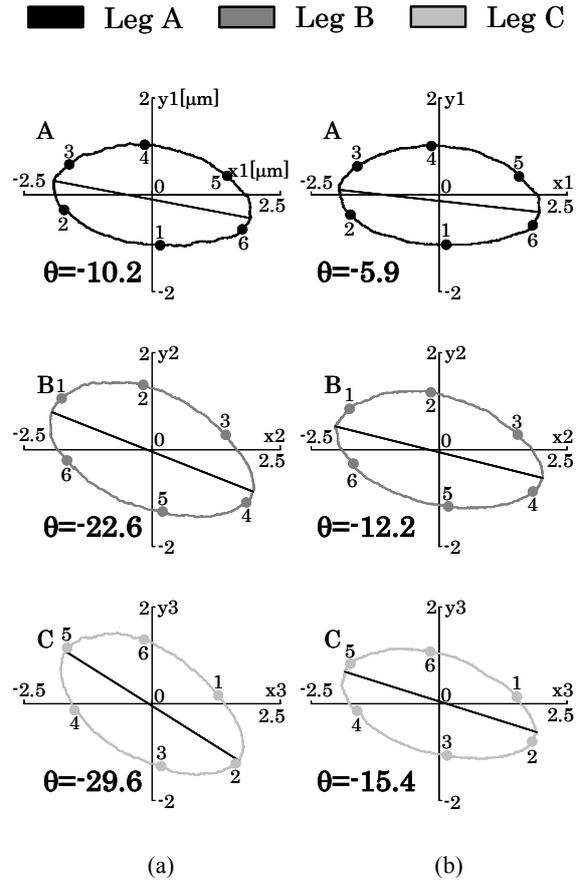
**Fig. 9** Three legs' trajectories in the local xy plane and the long axis angle  $\theta$ . The control waveform is sinusoidal. The direction is the CCW direction. The frequency is (a) 800 Hz and (b) 300 Hz.
