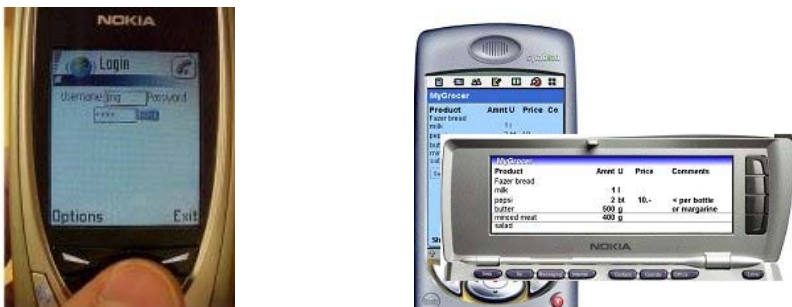
Fig. 8.2. Access to retail m-services via cellular wireless mobile devices: user authentication (left) and shopping list editing (right) on wireless enabled personal digital assistant and cellular mobile telephone (both Java 2 Micro Edition capable).
