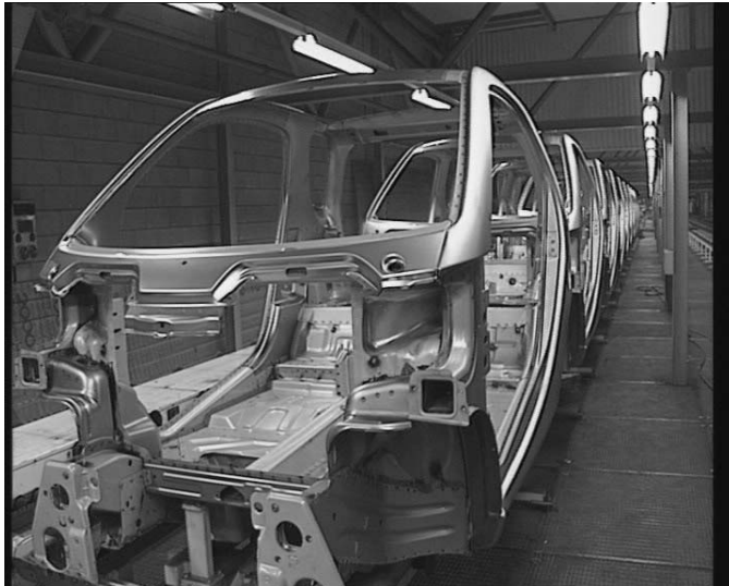
Figure 15.2. The Tridion safety cell, after complete assembly at smartville by a main ‘system partner’, Magna Chassis. Here, it is being conveyed to the main fortwo assembly line.
