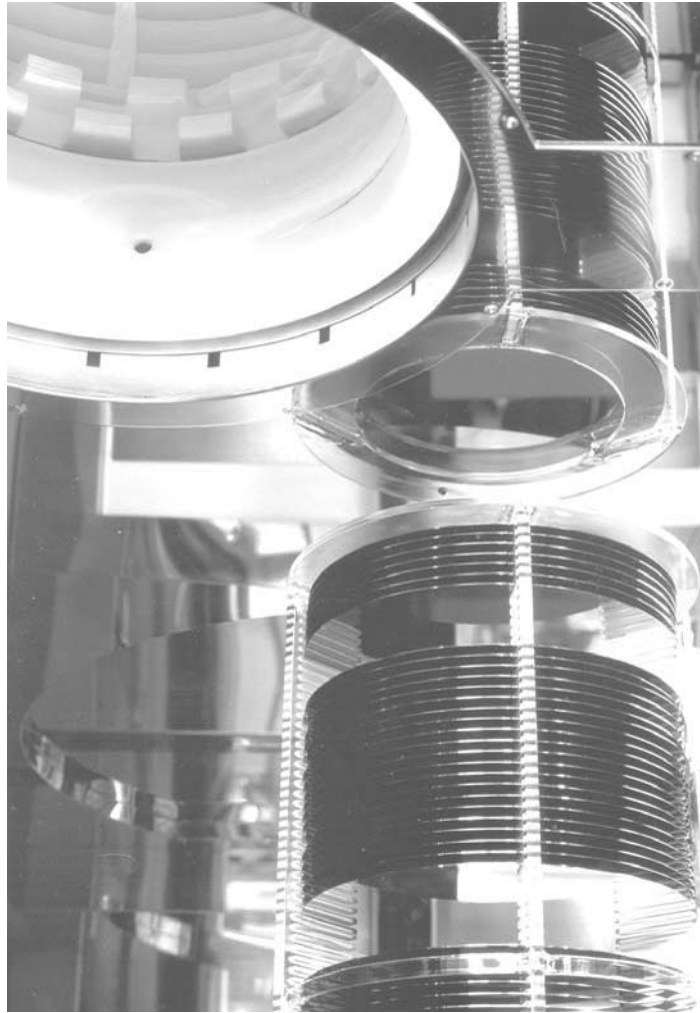
Fig. 2.3. Batched 300-mm wafers ready to go into a vertical furnace (open furnace tube on the upper left).
