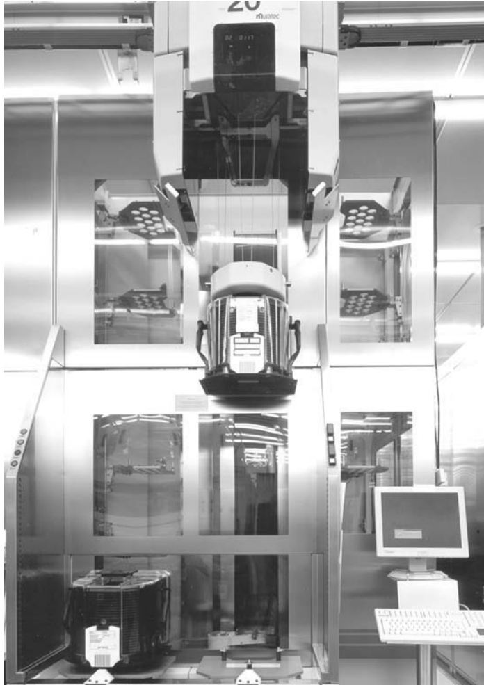
Fig. 2.5. Automatic transport system loading up a fully automatic wafer storage (Stocker).
