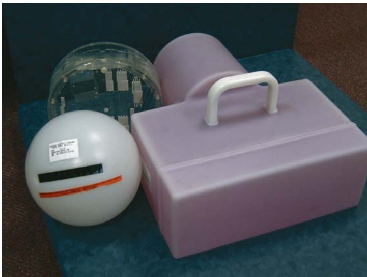
FIGURE 4.1. Selection of MRI test objects (left to right): 1.5 Tesla sphere, Eurospin TO4 (resolution), and a 3.0 Tesla head and neck phantom.
