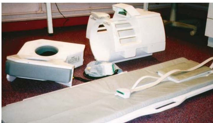
FIGURE 1.13. A selection of RF coils (bottom) pelvic-phased array, (top left) breast coil, and (top right) linear head coil.
