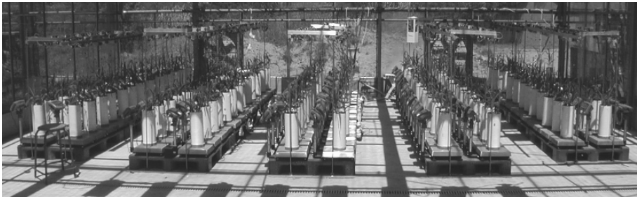
Figure 3. Phenotyping platform for continuous measurement of leaf elongation rate, soil water status and micrometeorological variables (up to 366 plants). Plants are grown in PVC columns and placed on balances. Each leaf is attached to a rotative displacement transducer. Environmental sensors (PPFD, vapour-pressure deficit, meristem temperature) are placed at plant level. All sensors are connected to data loggers with a time resolution of 15 min.
