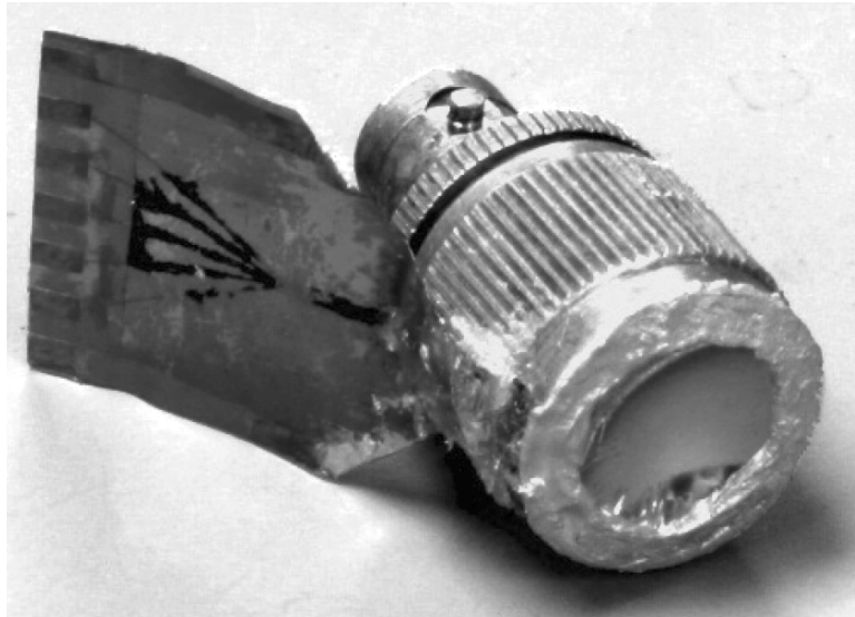
Figure 2. The annular array transducer mounted in an UHF connector. The UHF connector and PVDF membrane are electrically joined with silver epoxy.
