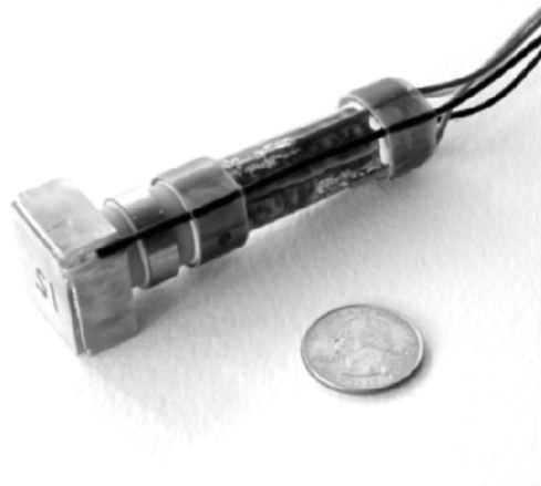
Figure 7. Push-pull, triple resonant Tonpilz transmitter transducer with co-located PVDF receiver.
