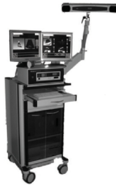
Figure 1. System prototype, including rf generator, ultrasound beamformer, personal computer and optical tracking device.
