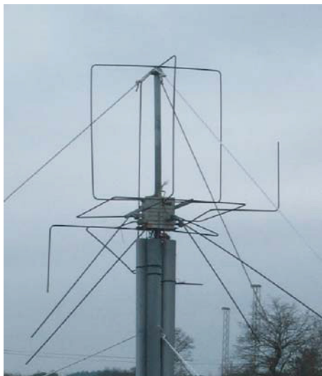
Figure 1. Array #1 of seven HF collocated antennas (patent n°99 16112)
