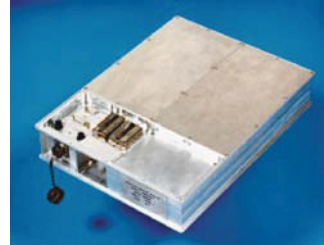
Cosmic Radiation Effects & Activation Monitor (CREAM) as installed onboard space shuttle, Boeing 747, executive jets, and Mir (Dyer et al. 1999; Dyer et al. 2005)
