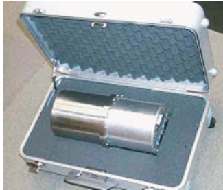
Tissue Equivalent Proportional Counter (TEPC, HAWK) installed on board Airbus A340, measurements on board space shuttle and Boeing 747 (Lindborg et al., 2004a; Beck et al., 1999b; Lindborg et al., 2004b)
