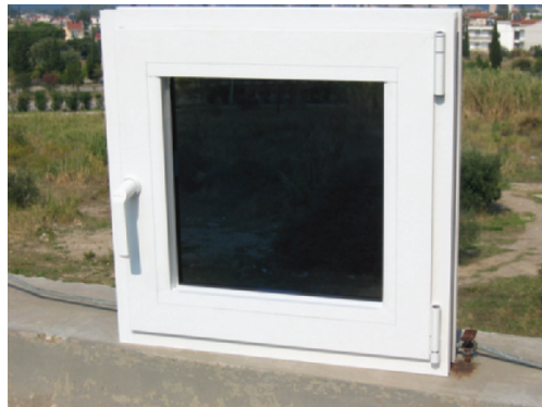
Figure 10.1 Electrochromic window prototype in the coloured state
