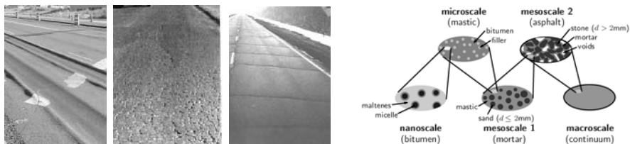
Figure: (left) failure modes in asphalt pavements and (right) multiscale model for asphalt
