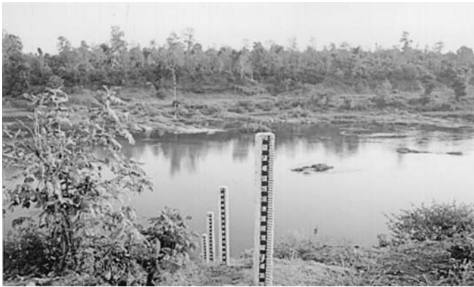
Figure 1. Sectional staff gauge
