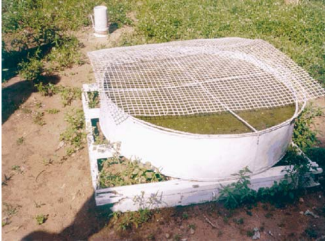
Figure 2. U.S. Weather Bureau class A land pan
