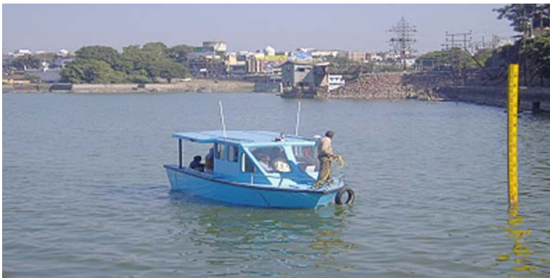
Figure 4. Measurement of discharge using moving boat method
