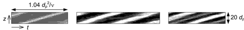
Fig. 3. Simulated space-time plots of the solids volume fraction. From left to right: \bar{\phi} = 0.580, 0.505, \text{ and } 0.488 .
