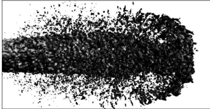
Fig. 8. The spatial development of an atomizing jet simulated in 3D (obtained by A. Leboissetier). The domain shown is 128 \times 128 \times 256 .
