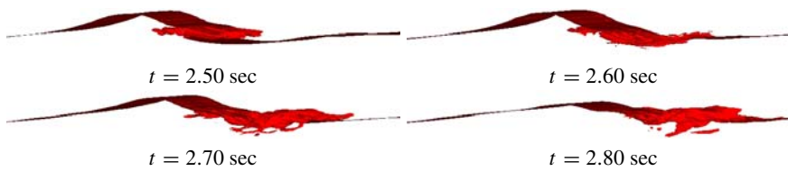
Fig. 2. Frames of C = 0.5 isosurfaces during a stronger plunging event.
