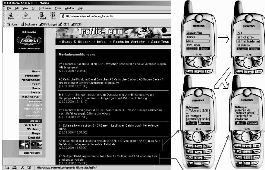
Figure 4: Sample of a traffic information page of an Internet WEB site of a public radio station: This source is used by the mining agent to collect the desired content - in the sample here the highway "A8" was defined as querying target. After launching the display MIDlet on the wireless terminal, the agent is activated by a HTTP query (containing as parameter the selected road), and the returned result is displayed. After this, the user can scroll through the response.
