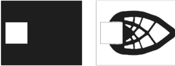
Figure 2. The initial configuration (full domain) and the solution obtained by the level set method with topological gradient.
